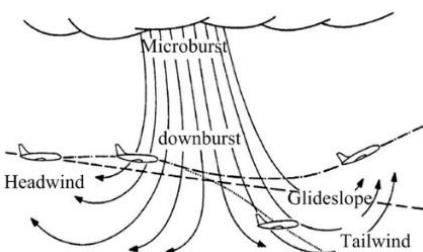
**Fig. 2** Aircraft encountering with microburst and deviating from the flight path.
