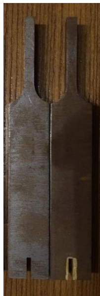
Fig.6 Fixtures made for fracture test
