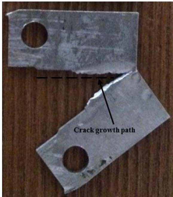
Fig.15 CT specimens after fracture test and crack growth path
