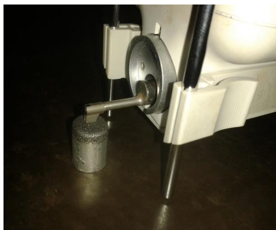
Fig. 3 Surface roughness Measurement after discharge operations
