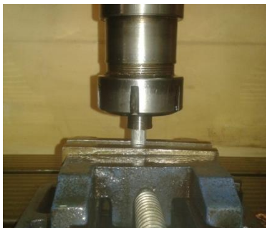
Fig. 2 Setting the electrode to electrical discharge process
