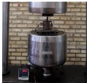
Fig. 3 Quasi-static hot pressing equipment using for powder compaction
