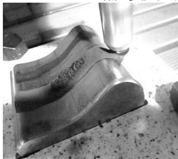
Fig. 25 remained powder on the work piece surface
