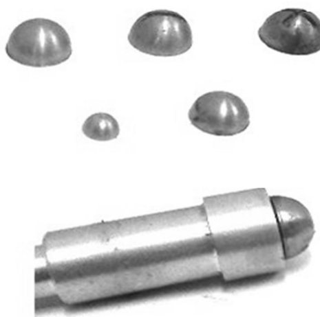
Fig. 2 Hemispheres made of 99.8% pure iron
