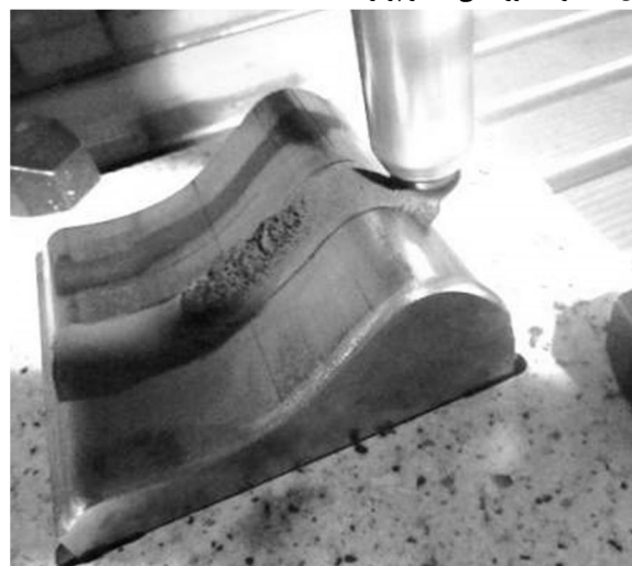
Fig. 25 remained powder on the work piece surface
