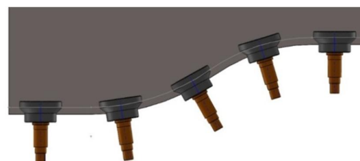
Fig. 6 The verticality of rollers in different positions on the bend curve
