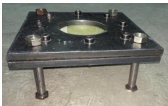
Fig4. Fixture of Punch shear test
