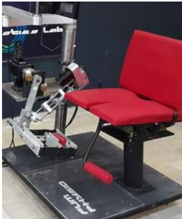
Fig. 6 FUM-Physio with FUM-LSEA as supplementary force source
