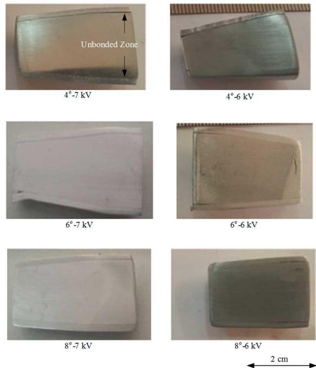
Fig. 6 Macroscopic images of section of weld samples
