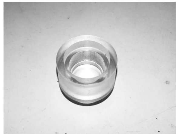
Fig. 4 Wedge made for the transmission of ultrasonic waves
