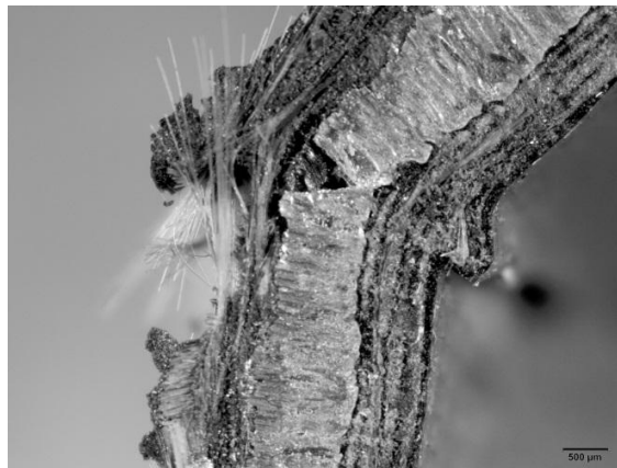
Fig. 5 Optical microscope image of the failed FMLs in the three point bending test
