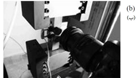
Fig. 1 The tensile test apparatus (a), clamped specimen with extensometer and a camera (b)
