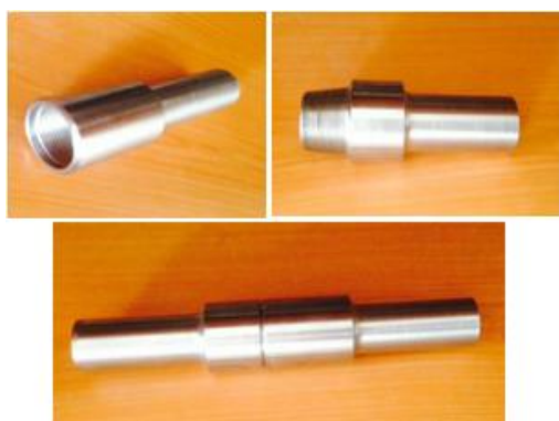
Fig. 3 Tool joints made in scale of 0.2
