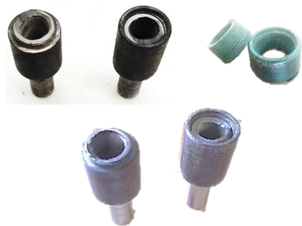
Fig. 21 Failure of tool joints after fatigue test
