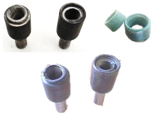
Fig. 21 Failure of tool joints after fatigue test
