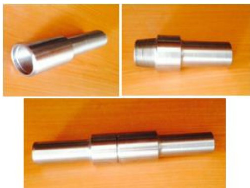
Fig. 3 Tool joints made in scale of 0.2
