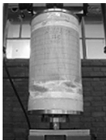
Fig. 7 Cylinder after buckling
