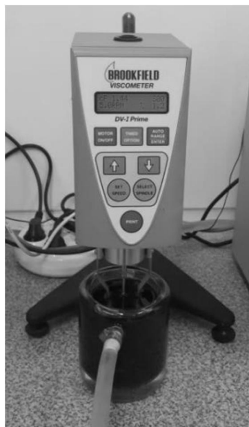
Fig. 2 Measurement of viscosity using Brookfield DV-1 PRIME digital Viscometer equipped with a temperature bath
