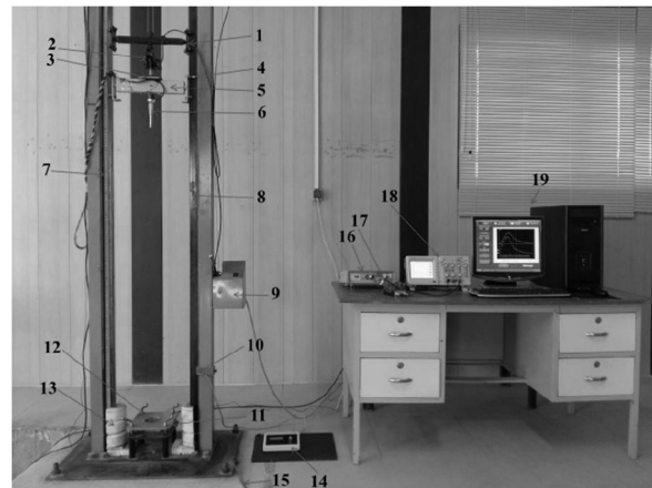
Fig. 15 A picture of the drop-weight impact testing machine and the data acquisition system (the experimental set up)
