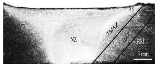
Fig. 4 Macrograph of FSPed sample showing the regions around the FSP zone
