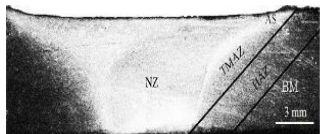
Fig. 4 Macrograph of FSPed sample showing the regions around the FSP zone
