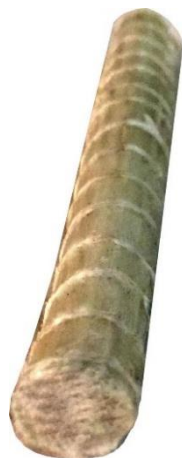
Fig 5. Pultruded rod with helically-wound fibers
