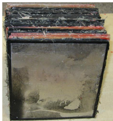
Fig. 3 Made samples with different percentages of carbon nanotubes
