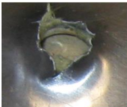
Fig. 8 Kevlar fiber tensile failure
