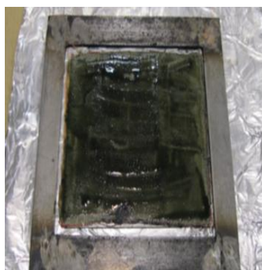
Fig. 1 Padding-hand samples of hybrid nano composites kevlar/ epoxy and aluminum
