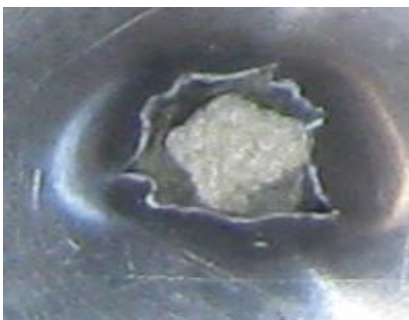
Fig. 10 The separation between the aluminum and kevlar fiber
