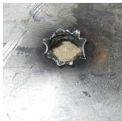
Fig. 7 Petaling phenomenon due to the conical bullet nanocomposite panel
