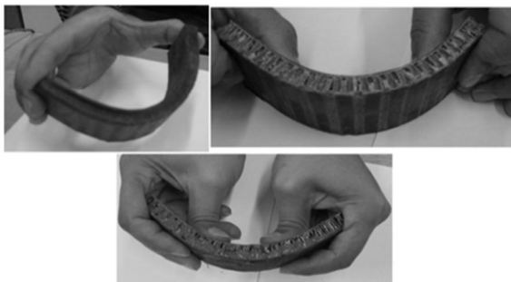
Fig. 2 Different flexibility of sandwich panel
