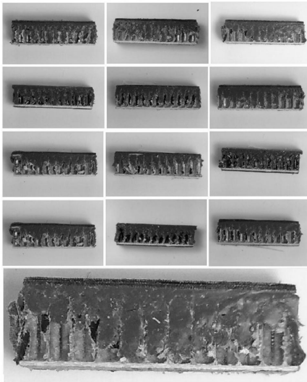
Fig. 15 Sections of flexible samples in the slot locations
