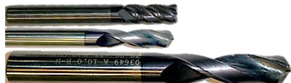
Fig. 1 Tungsten carbide flat end mill and drill bits with diameter of 6 and 10 mm used in tests
