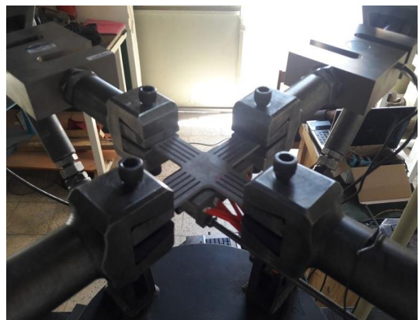
Fig. 3 The method of fixing a cruciform specimen based on the dependent biaxial tension mechanism
