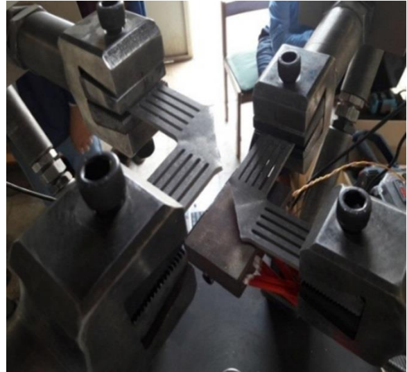
Fig. 8 The cruciform specimen fracture from Al. alloy 5083
