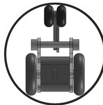
Fig. 1.b Conceptual design of the robot, Front view
