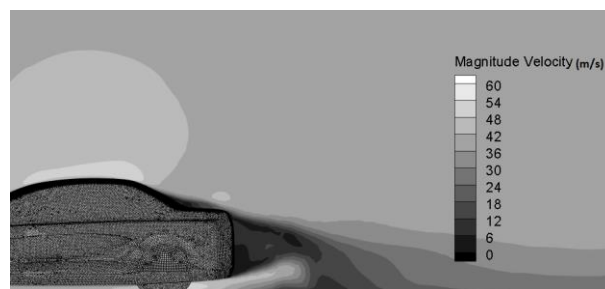
Fig. 17 distribution of velocity on the simple model
