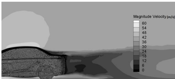
Fig. 20 distribution of velocity on the model with spoiler and Curvature of lateral surfaces
