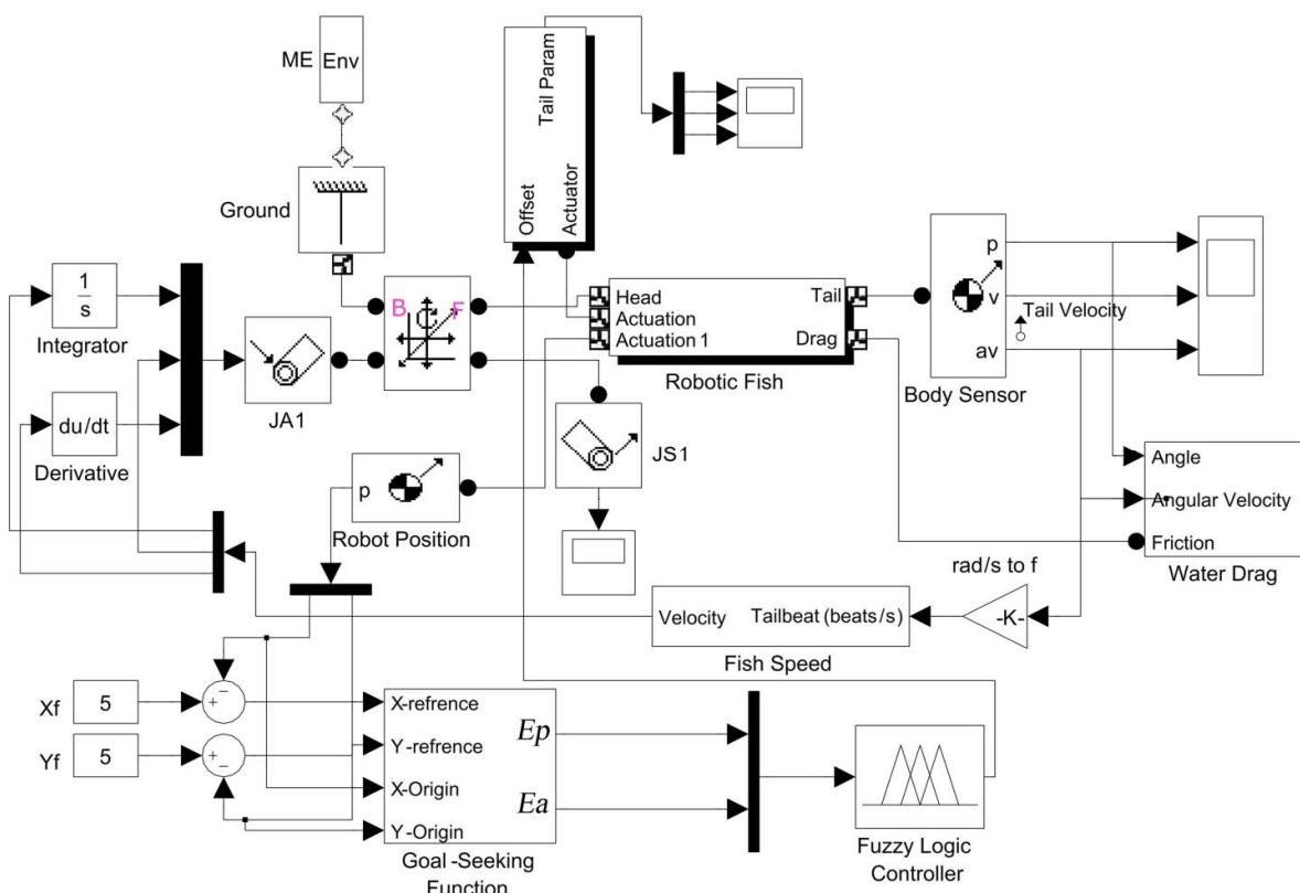
Fig. 10 Closed-loop configuration of the robotic fish in MATLAB software
