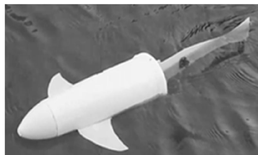
Fig. 6 Prototype model of the robotic fish in experimental environment
