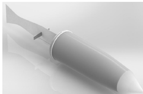
Fig. 5 3D virtual model of the robotic fish in Solidworks
