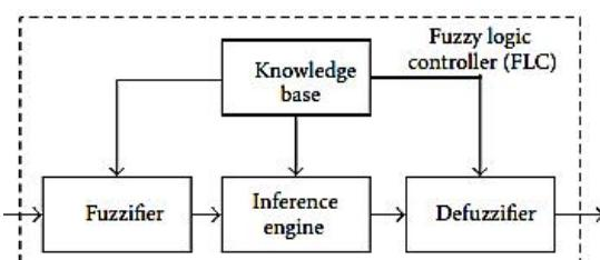
Fig. 7 Architecture of a basic fuzzy logic controller
