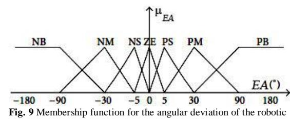
Fig. 9 Membership function for the angular deviation of the robotic fish
