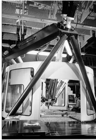
Fig. 3 a sample of octahedral machine manufactured by Ingersoll company
