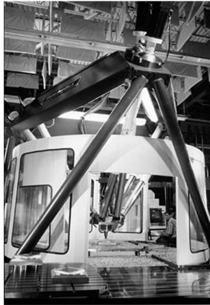
Fig. 3 a sample of octahedral machine manufactured by Ingersoll company
