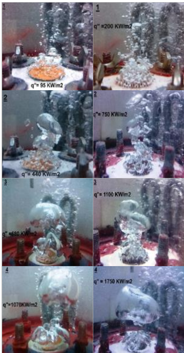
Fig. 17 Image of comparison of bubbles formation in flat plate and micro channel
