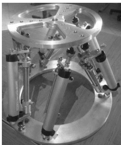
Fig. 1 The 6-DoF pneumatically-actuated HexaTaar robot
