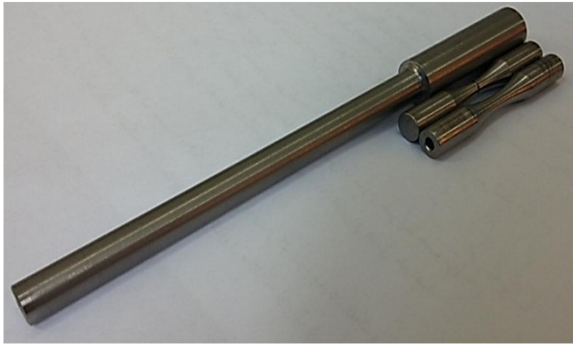
Fig. 4 Specimens used for fatigue tests
