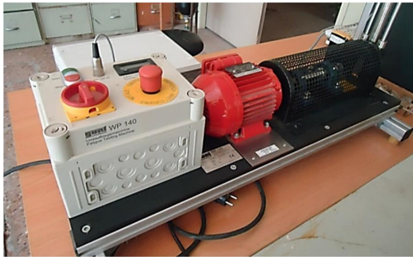
Fig. 5 Rotating Bending fatigue machine
