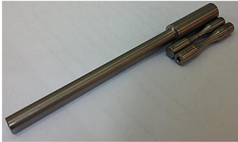
Fig. 4 Specimens used for fatigue tests
