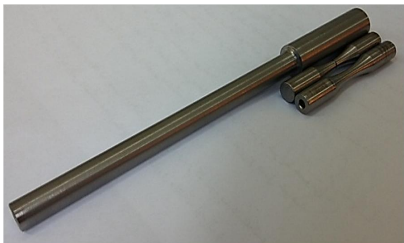
Fig. 4 Specimens used for fatigue tests
