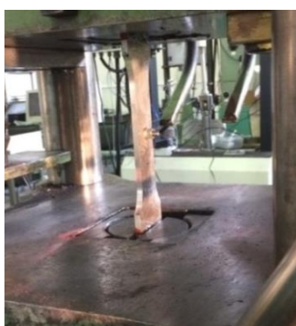
Fig. 6 Test specimen mounted on the fatigue test machine
