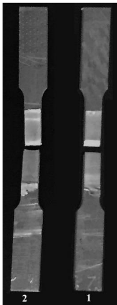
Fig. 7 Tensile test samples after fracture (sample 1 and 2 of Table 2)
