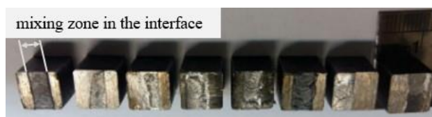
Fig. 12 Fracture surface samples tensile shear test
