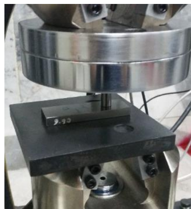
Fig. 5 Setup of press fitting the pin into the steel specimen hole
