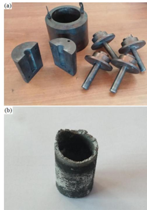
Fig. 2 (a) Designed mold and (b) Extruded part
