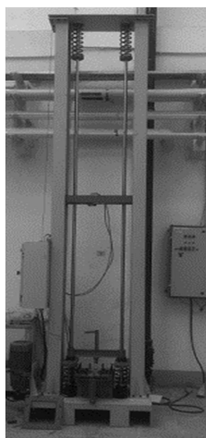
Fig.3 Low velocity impact device
