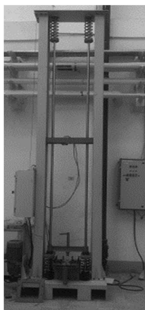
Fig.3 Low velocity impact device
