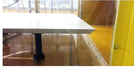
Fig. 7 View of the leading edge of the table which is designed sharply
