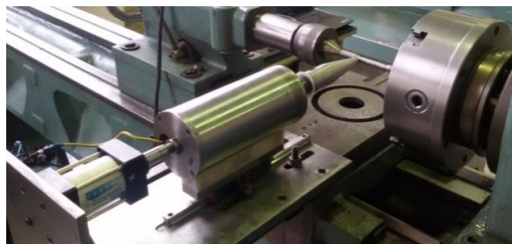
Fig. 10 Assembling of UPT equipment on the lathe
