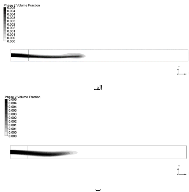
Fig. 6 Contours of volume fraction in the center plane at t = 1.4 s a) with considering diffusion effect b) without considering diffusion effect
