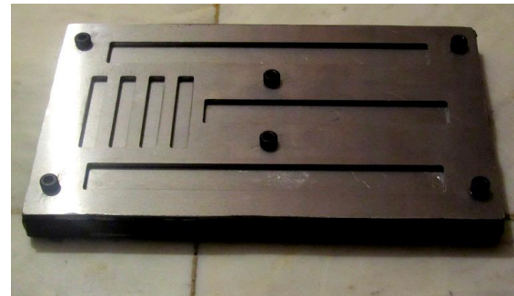
Fig. 3 Fabricated mold for samples of tensile, flexural and impact
