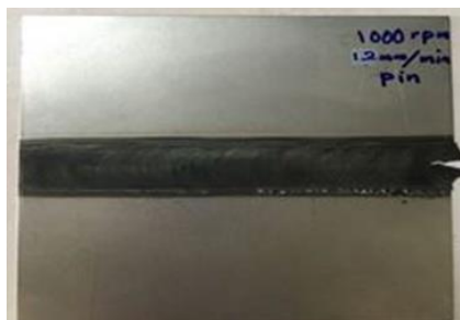
Fig. 3 The welded specimen with rotational speed of 1000 rpm and feed rate of 12 mm/min
