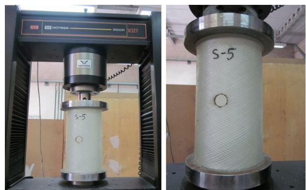
Fig. 6 A specimen prepared for buckling test
