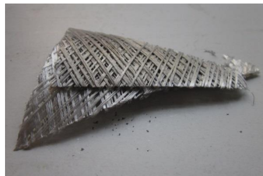
Fig. 4 A part of the shell which is burned to determine volume fraction of fiber in the shell
